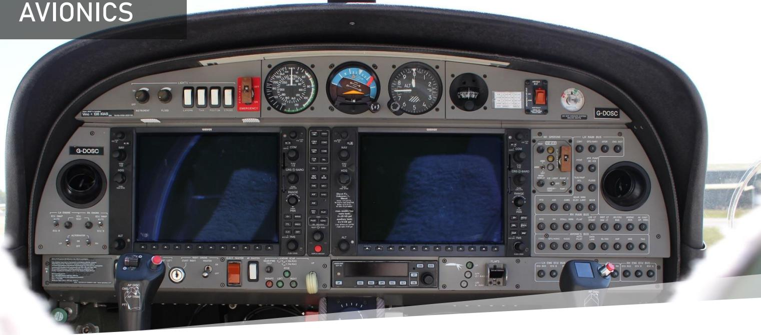
Diamond Aircraft selected the Garmin G1000 integrated avionics system for the DA42 Twin Star.
